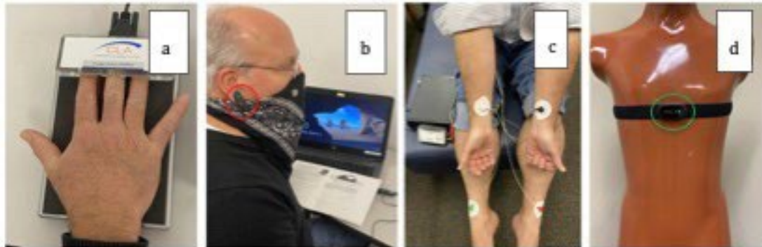
Figure 1. Equipment connections for Heart Rate Variability (HRV) devices a) CLA INSiGHT, b) emWave2 ear sensor (red circle), c) iWorx, and d) Polar H10 (green circle - ECG sensor).
