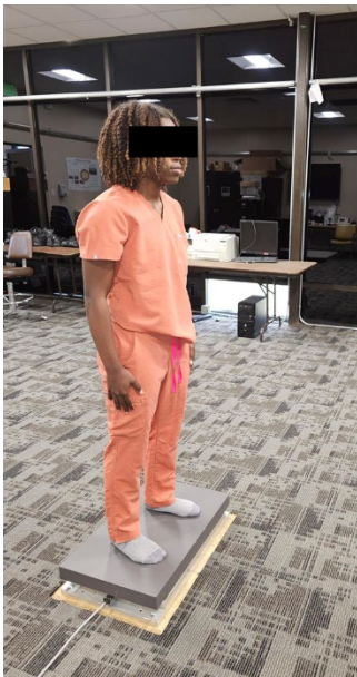
Figure 2. Image of a participant having their balance analyzed for 30 seconds eyes-closed on a force plate. Participants removed their shoes and stood with their feet shoulder-width apart and their arms at their side as still as possible.
