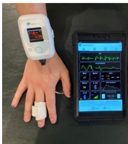
Figure 7: Caretaker 4 equipment (i.e., wireless wrist monitor, finger cuff, tablet) and set up.
