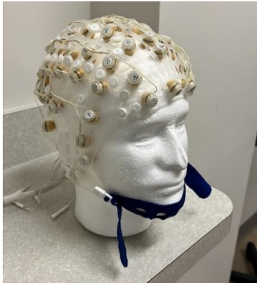
Figure 3: 64-channel Quik-Cap Hydro Net
